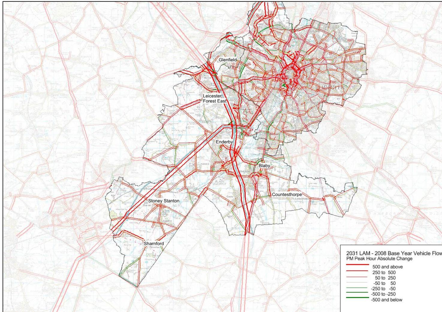
Figure 5.7: PM Peak Hour Absolute Vehicle Flow Changes: 2031 'Hard' Only – 2031 LAM
