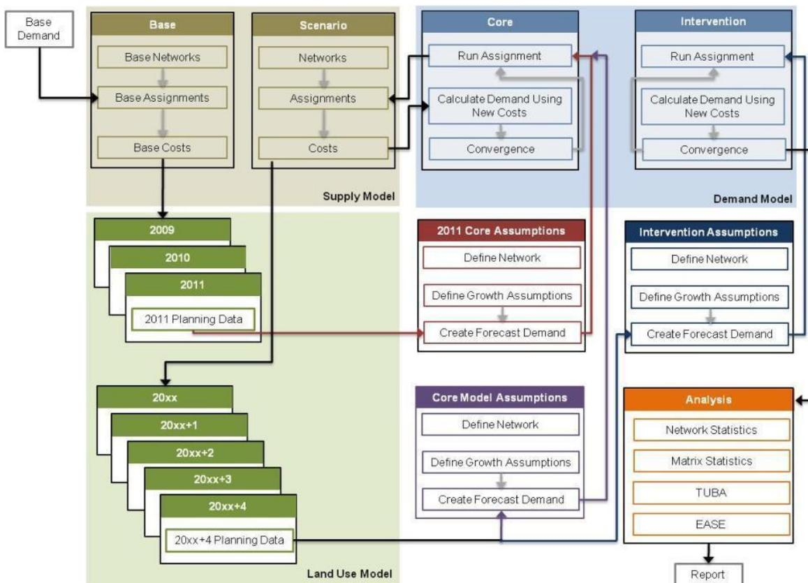
This shows the flow of information required in building up a core scenario, with costs from previous years being used in the land-use model, which in turn then allocates growth in the subsequent years. Trip growth is calculated by applying a customised version of the DfT’s trip-end model to the planning data generated in LLITM-LUM. This means that the core scenario years need to be run in sequential order, with the output from one forecast year forming some of the inputs for the next.
