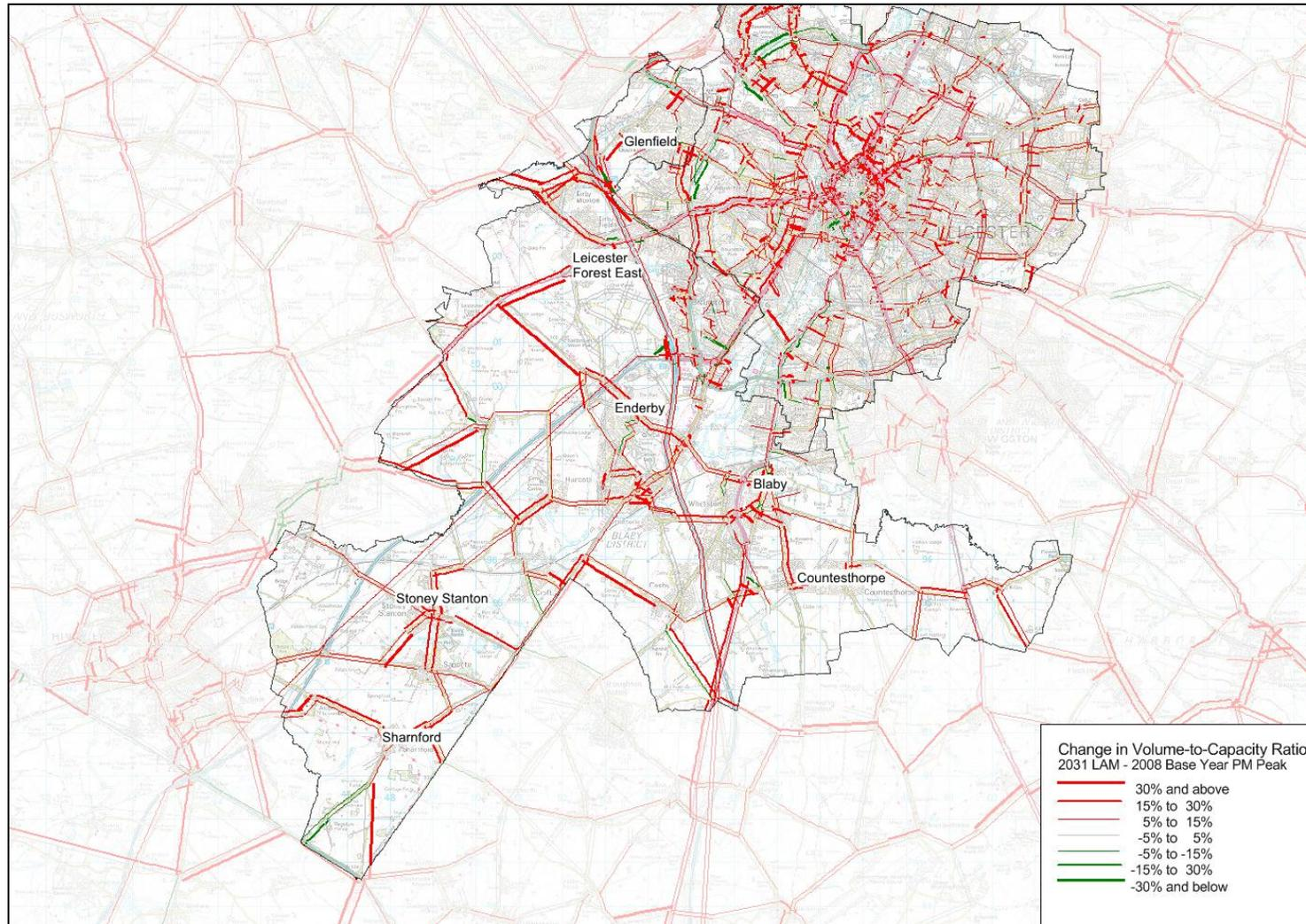
Figure 5.14: 2031 'Hard' Only - LAM PM Peak Hour Volume-to-Capacity Ratios
