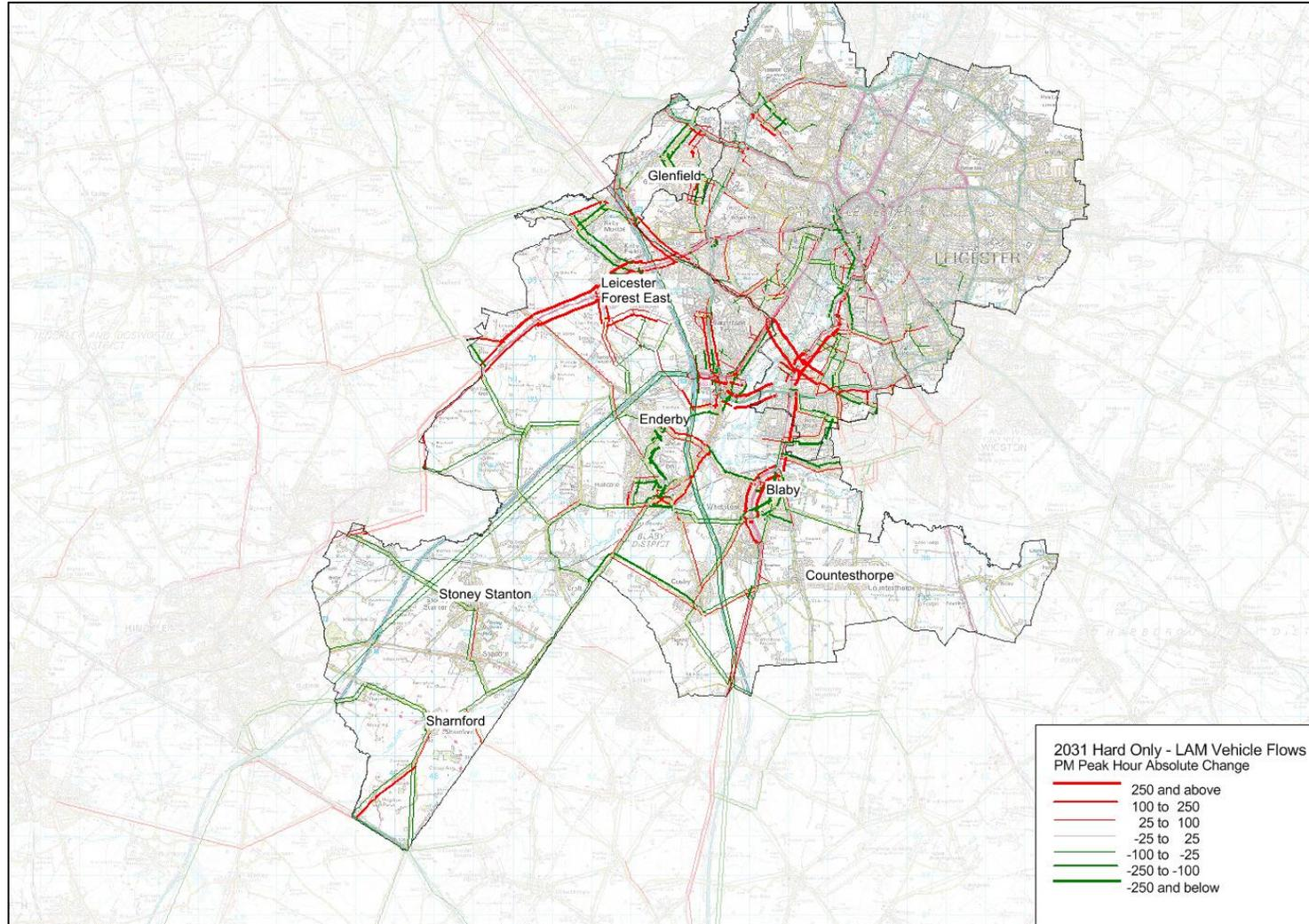
Figure 5.8: PM Peak Hour Absolute Vehicle Flow Changes: 2031 Mitigation – 2031 LAM
