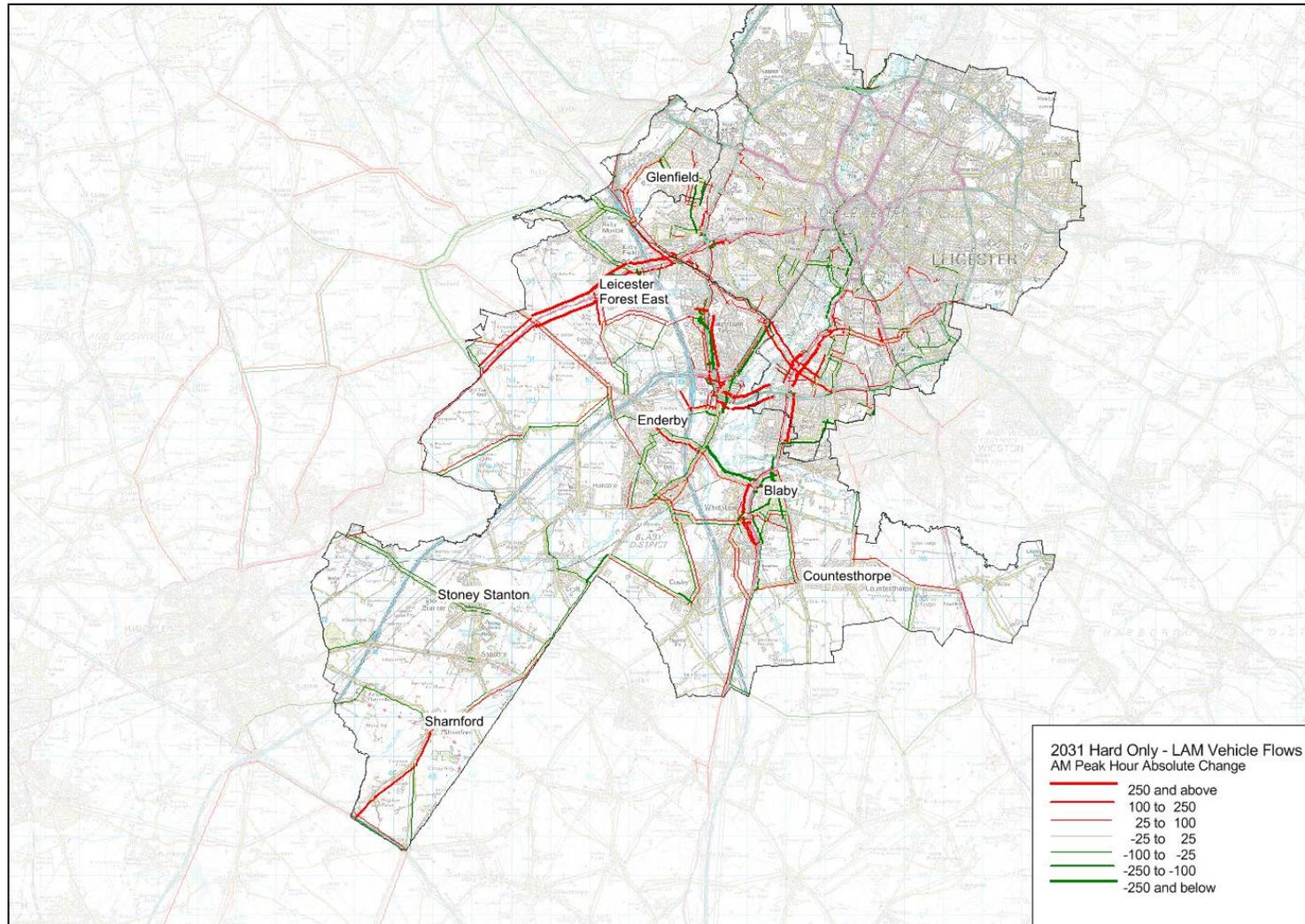
Figure 5.4: AM Peak Hour Absolute Vehicle Flow Changes: 2031 Mitigation – 2031 LAM
