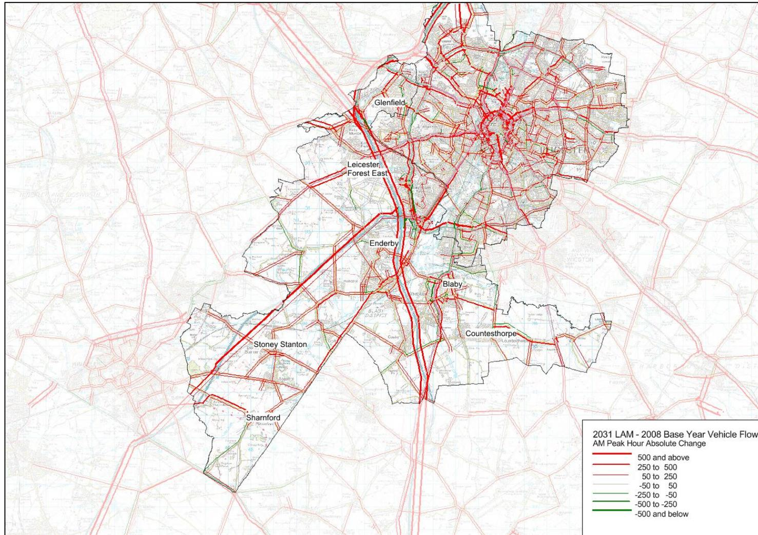
Figure 5.3: AM Peak Hour Absolute Vehicle Flow Changes: 2031 'Hard' Only – 2031 LAM
