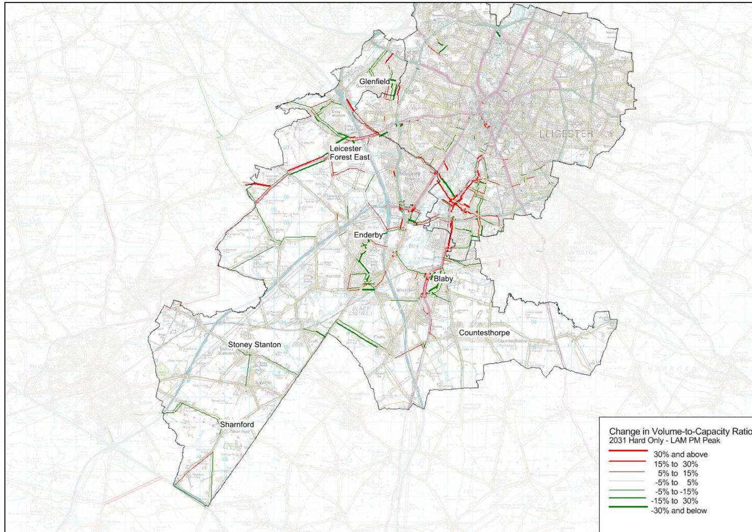
Figure 5.15: 2031 Mitigation - LAM PM Peak Hour Volume-to-Capacity Ratios
